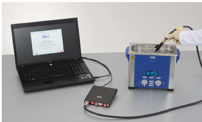
Elmasonic P 30 H during the cavimeter test
